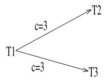
Indeed, a priori, we can start  $T_2$  and  $T_3$  at the same time. Indeed, it is either  $T_3$  is on the same processor as  $T_1$  and then  $T_2$  must wait 3 seconds communication or vice versa is that  $T_3$  must wait.
