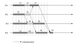
It may be noted that this algorithm gives an allowance of 4 processors while the width of the graph is 3.
