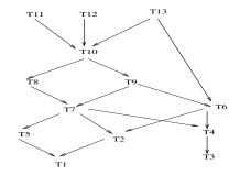
For example, T6 and T7 are the same "level". As  $succ(T_6) \subset succ(T_7)$ , T7 will be a priority. Intuitively, performing  $T_7$  before  $T_6$  was more likely to allow the continuation of dependent tasks of  $T_7$  that do not depend to  $T_6$ : Example  $T_5$ .
